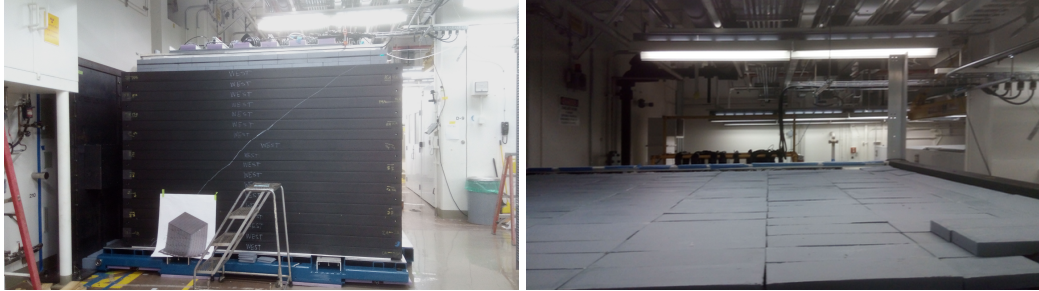
Figure 2.18: (left) High density polyethylene shielding assembled in a log cabin style around the detector. (right) layer of lead bricks situated on top of the detector.
