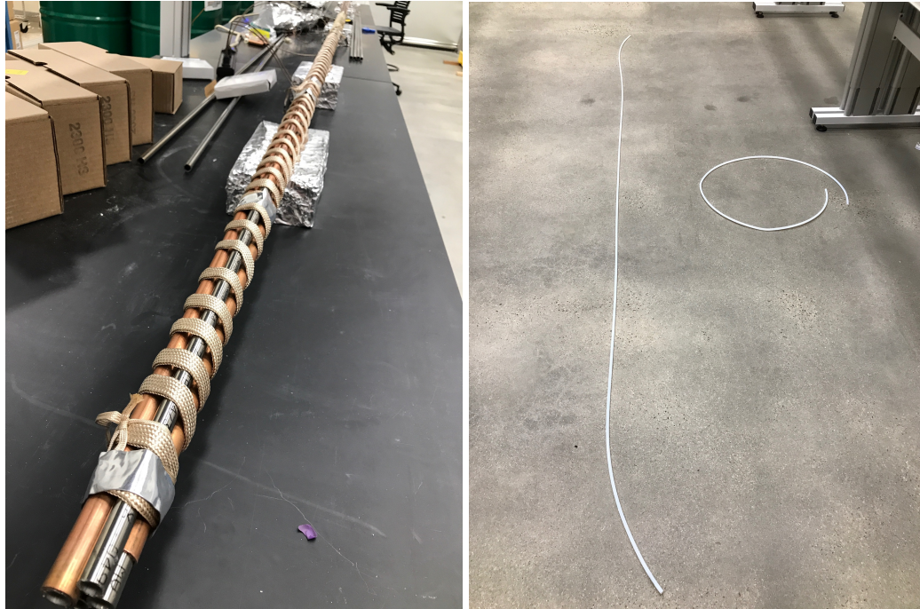
Figure 2.21: (left) Setup of the Oven for the Annealing of Teflon (OAT) used to prepare the PTFE tubes for the PROSPECT source calibration system. Heater tape, operated by a controller with two K-type thermocouples mounted inside the insulation (not shown), was wrapped around tubes of copper and stainless steel with an inner diameter matched to the outer diameter of the PTFE tubing. (right) Photograph showing the different behavior of the initial curved tubing and the straightened, annealed tubing.
