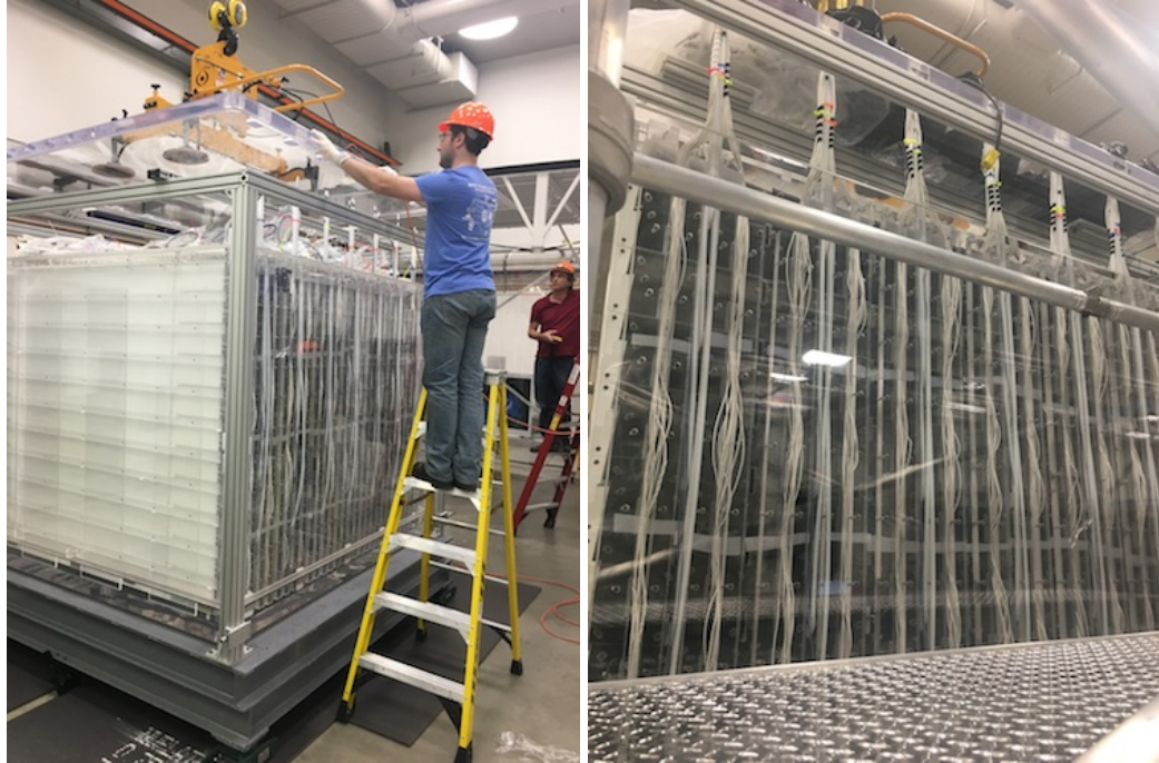
Figure 2.16: (left) Photograph of the acrylic lid being lowered onto blocks on top of the acrylic sidewalls. (right) After blocking up the lid, cables and PTFE calibration tubes were fed through the holes in the lid. Then the blocks were removed, and the lid was lowered down onto an FEP strip along the rim of the side walls.
