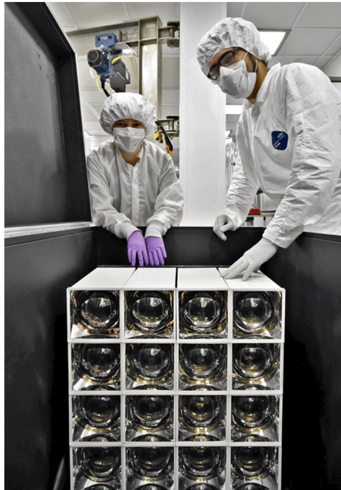
Figure 2.12: One of two dark boxes used to test batches of 16 PMTs for the PROSPECT detector.
