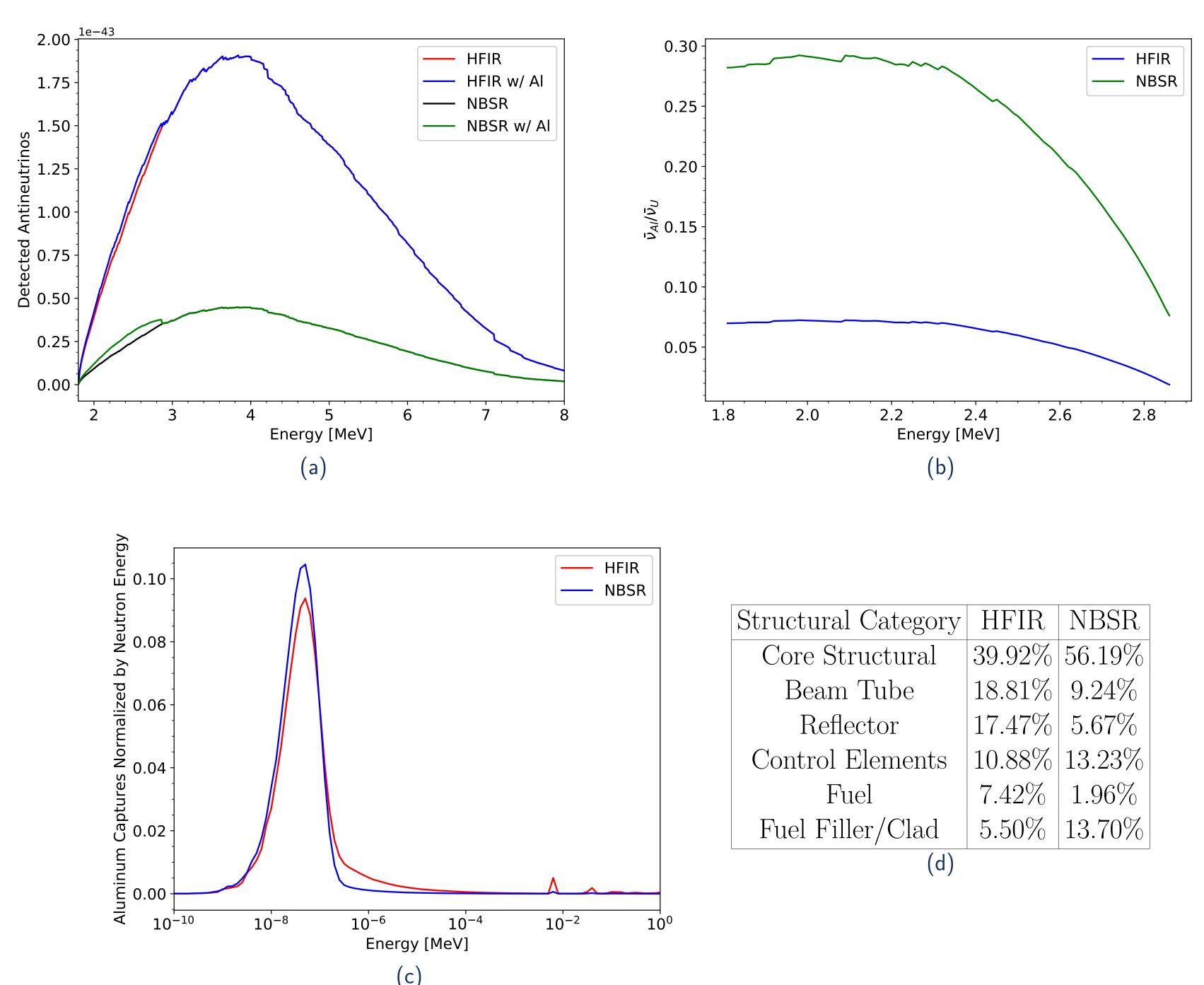
Figure 7: Comparison of antineutrino spectra from HFIR and NBSR with and without aluminum activation (a), the non-fission excess antineutrinos aluminum contributes (b), and energy spectra and regional distribution of aluminum captures in both cores (c,d)
