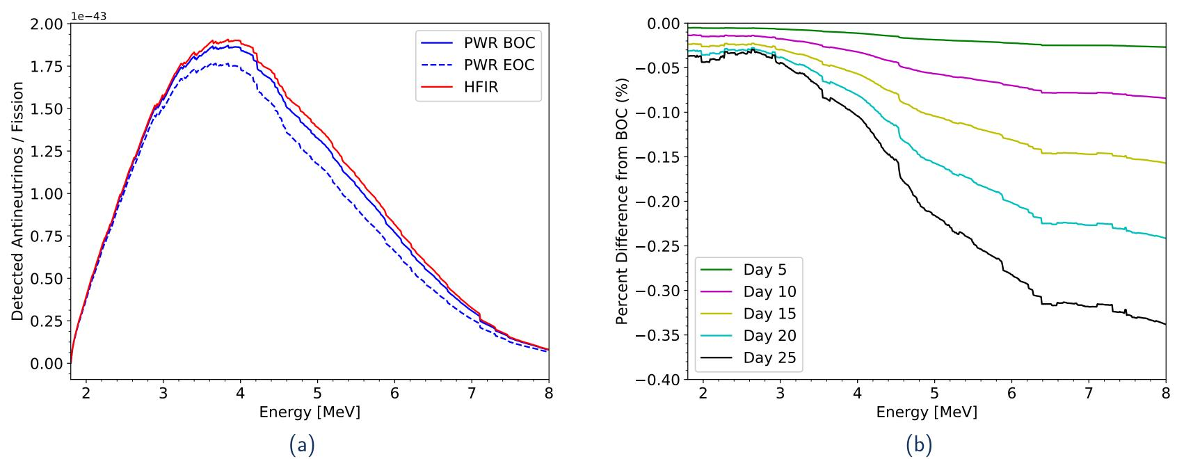
Figure 6: Spectra of detected antineutrinos per fission for the beginning and end of cycle for a PWR compared to that of HFIR (a) and the percent difference in each energy bin for HFIR relative to beginning of cycle (b)
