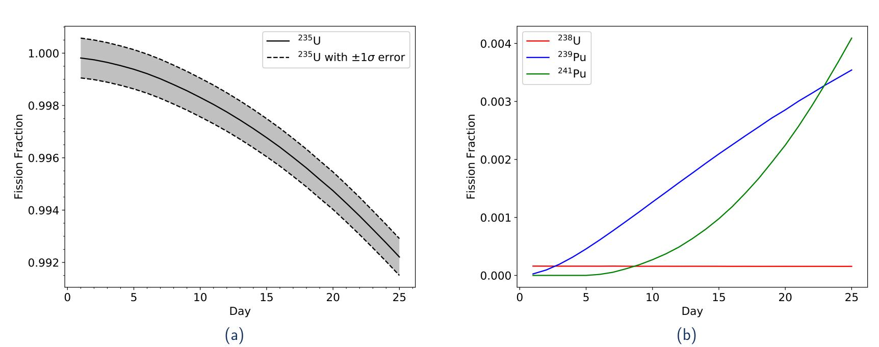
Figure 5: Fission fraction of <sup>235</sup>U by day in the HFIR cycle (a) and for the other three fissile isotopes (b). Note that error bars are not shown for the latter due to being small compared to the data
