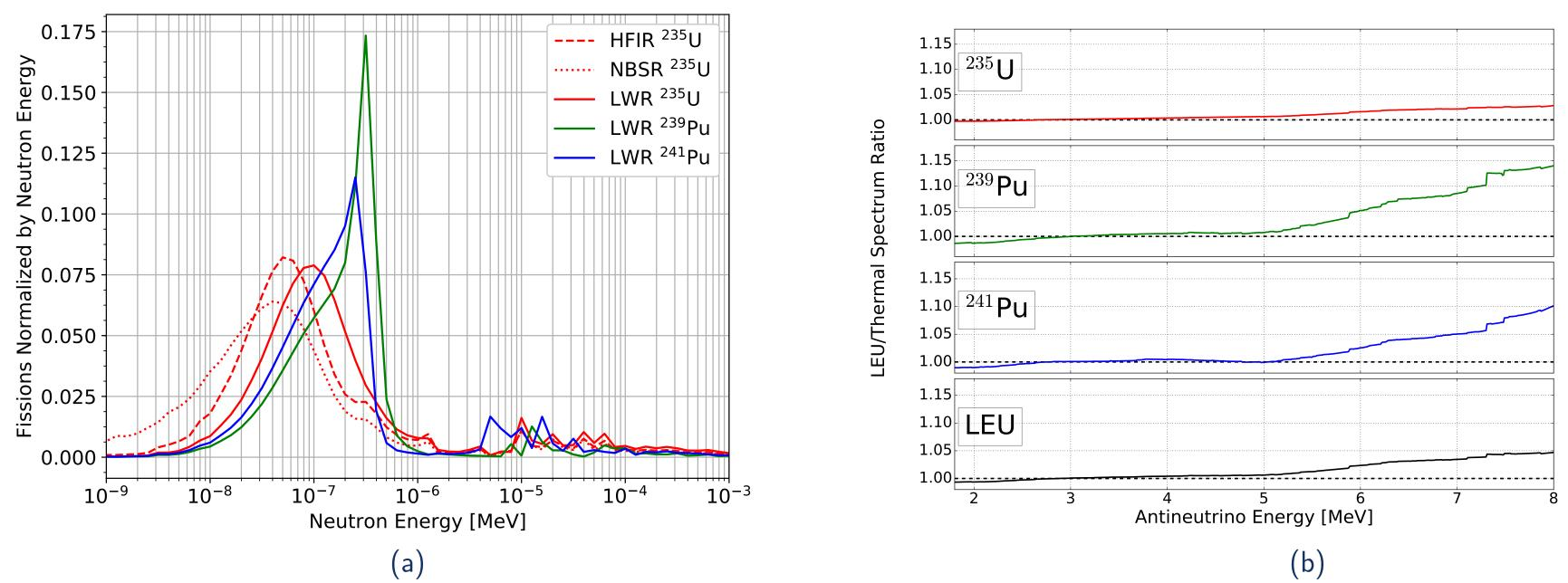
Figure 8: Energies of fission inducing-neutrons (a) and the propogation of that uncertainty to antineutrino spectrum differences compared to that of a PWR mixed spectrum (b) [12]
