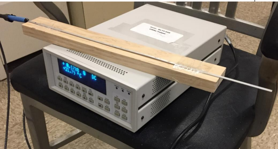
HMMT-6J18-VF hall probe connected to a Lakeshore 475 DSP gaussmeter
