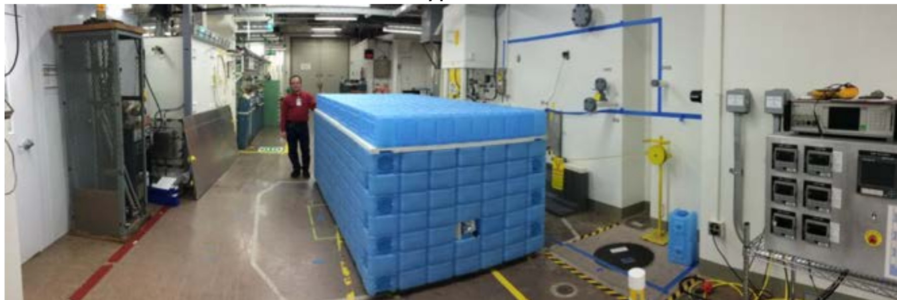
PROSPECT20 Prototype in Shield at HFIR
