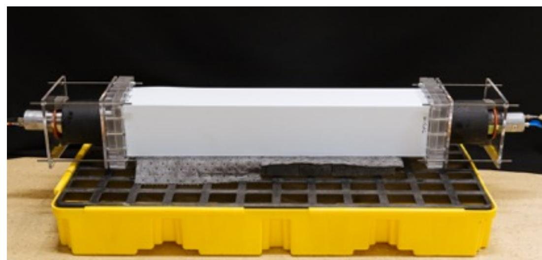
Detector geometry: 23L 1-meter rectangle
