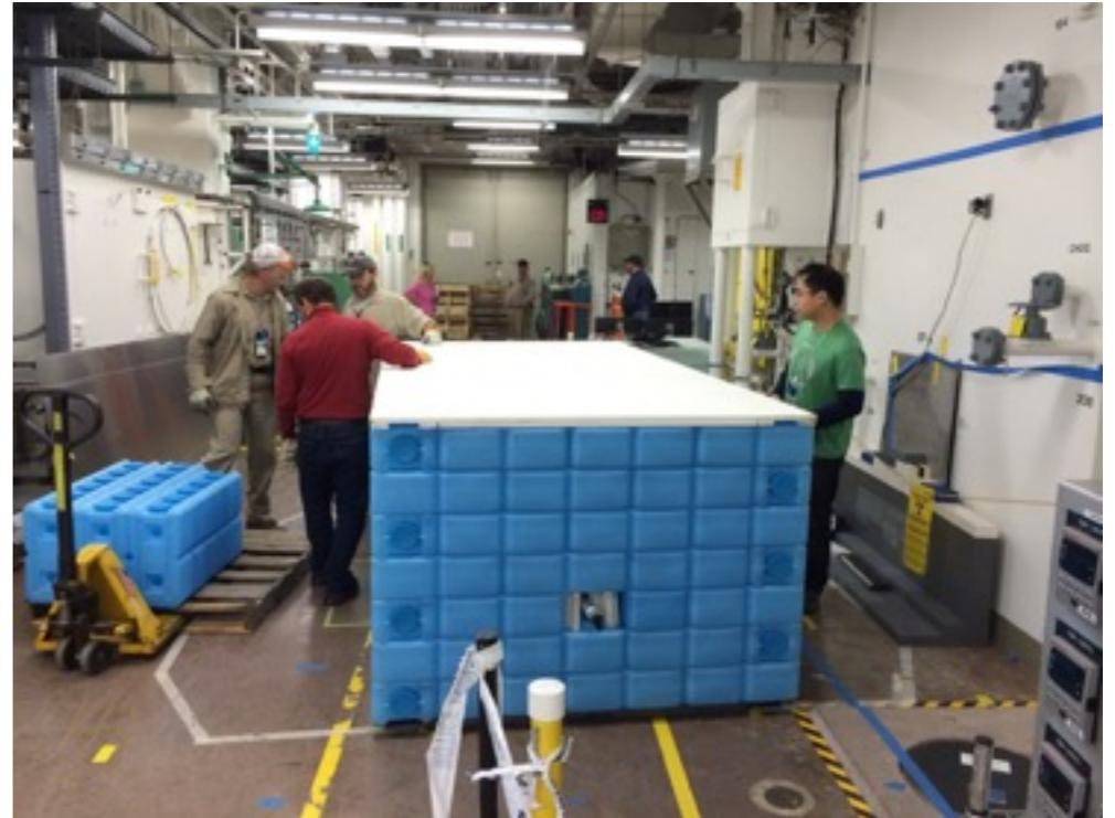
Detector geometry: 23L 1-meter rectangle
