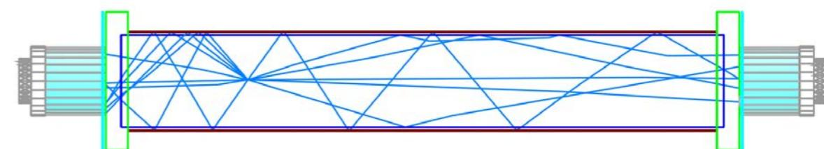
simulation of PROSPECT-20 with optical transport
