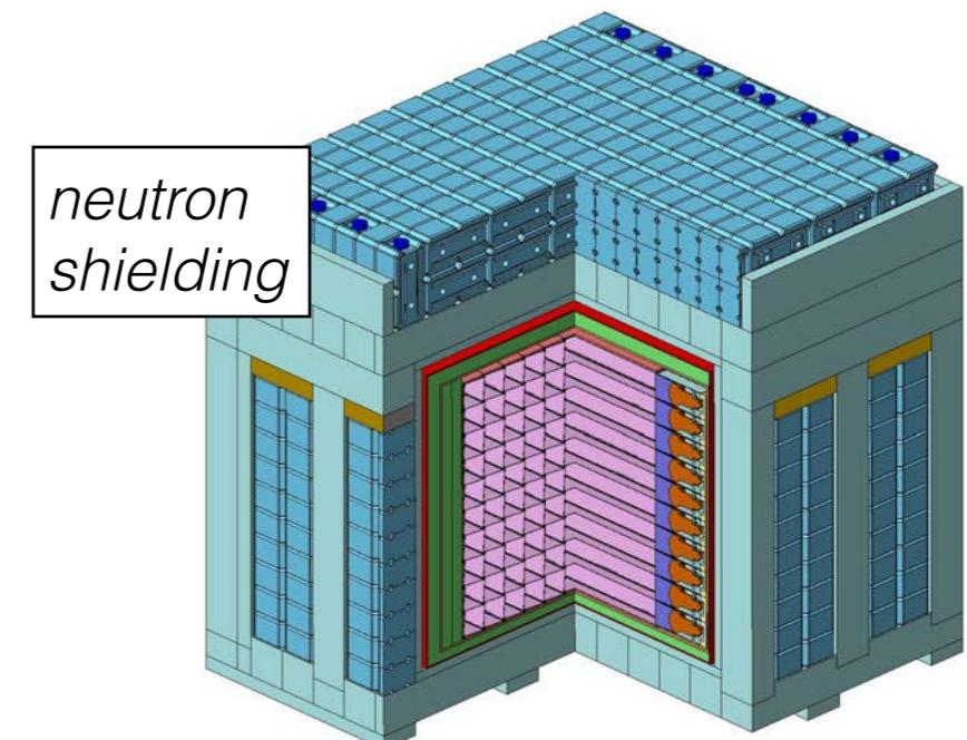
**detector structure and passive shielding designed for near-surface backgrounds**
