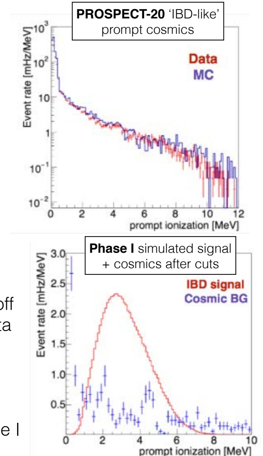
**prototype deployment validated background MC to project Phase I S:B**
