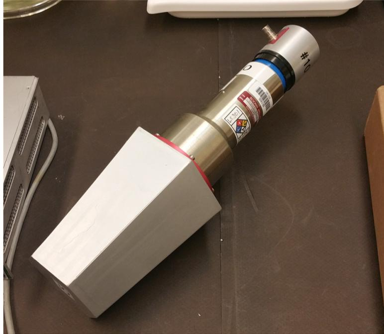
FIGURE 4.10: Image of NE213 fast neutron detector as used on DANG.
