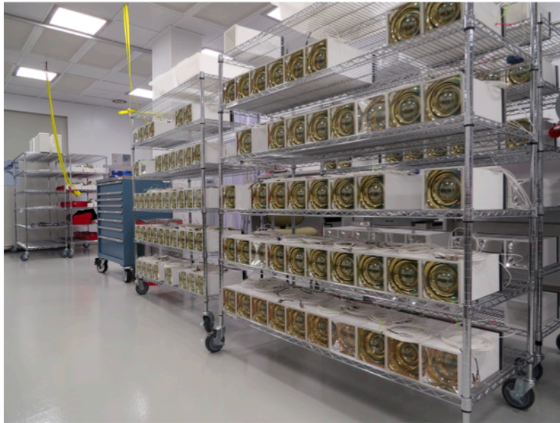
Figure 3.16: Rack of modules, some completed, others missing the PMT and/or mineral oil. The conical reflector can be easily seen in the empty acrylic enclosures.
