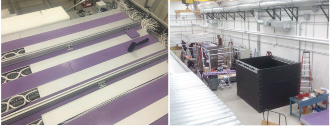
Figure 4.21: (left) Top of the detector package after cable routing. Lids to cable raceways and BPE strips are installed to create a flat surface for shielding to rest on. (right) Photograph of the exterior shielding package (black) construction, next to detector assembly.
