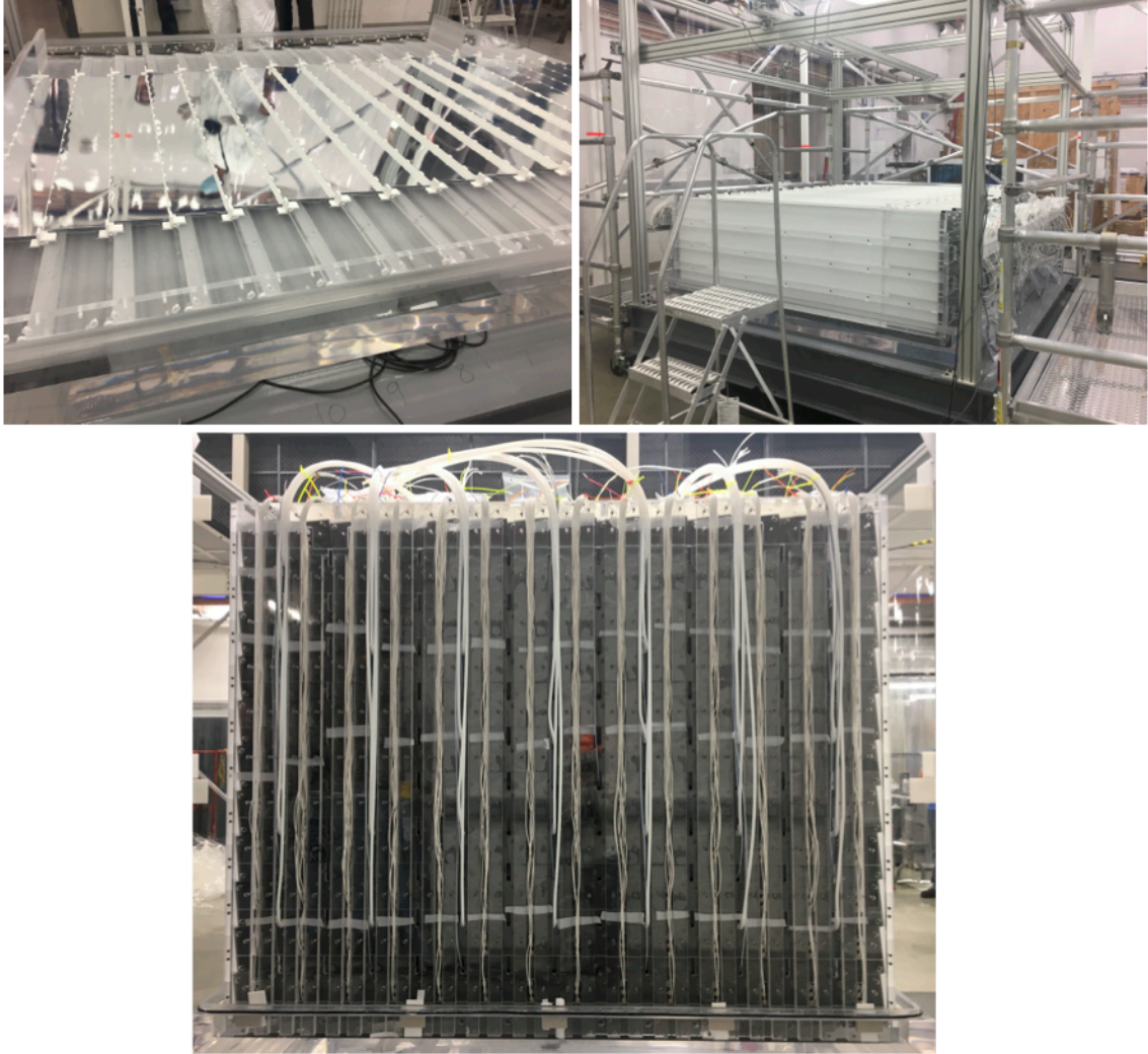
Figure 3.18: Photographs of the acrylic support system. (top left) Reflective separator and support rod assemblies installed on top of the bottom wedge planks. Two horizontal planks are also installed upright on either end. Horizontal PMT module support slats can be seen where the bottom planks terminate. (top right) Horizontal planks (clear) installed after four segment layers, defining the exterior of the optical grid. (right) Vertical and horizontal slats are bolted to the PMT modules to secure their position. They also serve as guides to route the cables and calibration tubes out of the detector.
