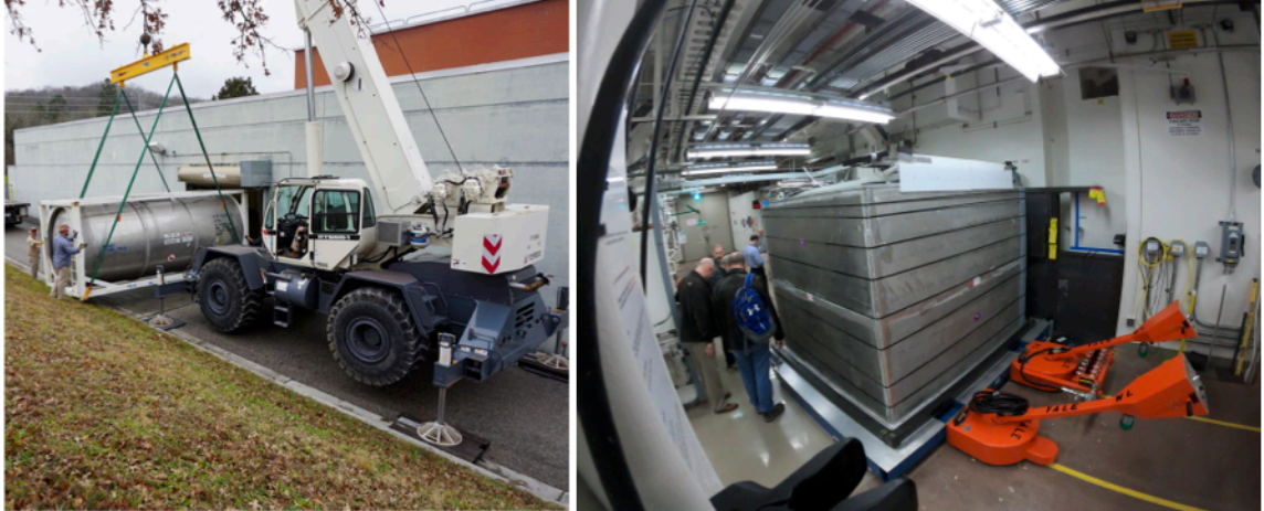
Figure 4.23: (left) ISO tank holding {}^6\text{LiLS} transported outside the HFIR building. The tank is significantly larger than required, but was recycled from a previous experiment. (right) Fisheye view of the detector package and chassis after being moved into Position 1 by the air casters and air drive motors (orange) [108].
