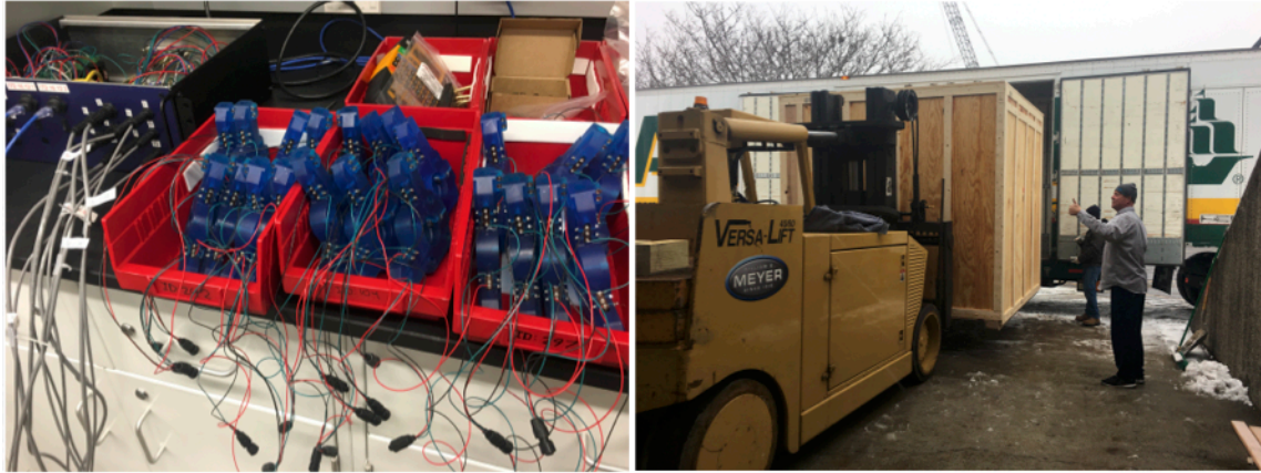
Figure 4.22: (left) 3D-printed pulley assemblies for the radioactive calibration drive motors after installation of electronics. (right) Detector packaging lifted onto a truck at the Yale Wright Laboratory for delivery to Oak Ridge.
