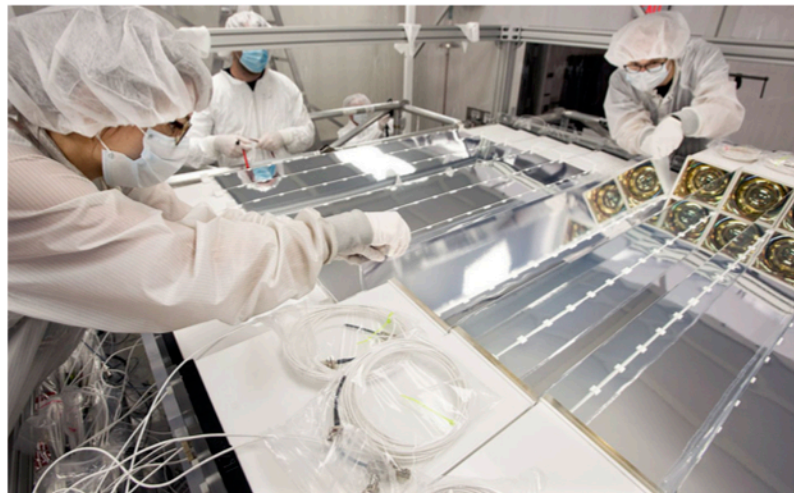
Figure 4.18: (top) Performing QC measurements on the last built layer. A motorized laser gauge is mounted on a linear slide rail spanning the width of the detector to measure the vertical profile of the reflective surfaces. Two different laser-cut aluminum gauges (one pictured) in combination with plastic feeler gauges are used to measure the profile of the PMT module back plugs and the end support rods that rest on the front window. (bottom) Detector assembly midway through the top row. A vertical optical separator is inserted into the support rods (white tabs) and PMT modules of previously installed layer. The white PMT module bodies and clear front windows are visible on the near side while the far side shows the PMT faces and conical reflectors. Photograph taken by Mara Lavitt.
