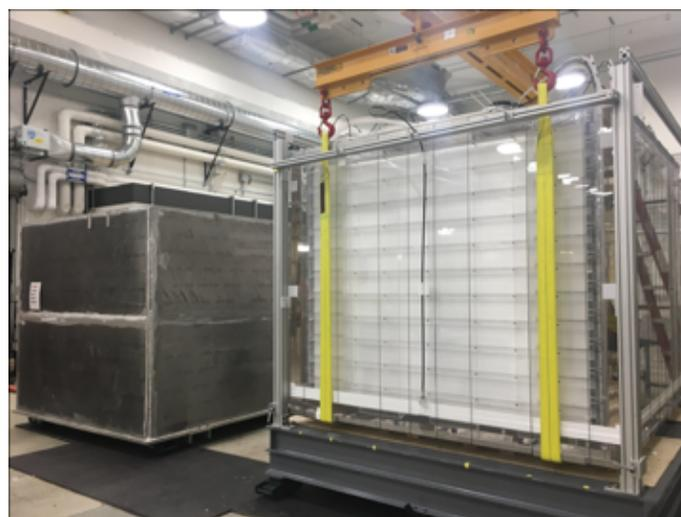
Figure 4.22. The aluminum (left) and acrylic (right) tanks as containment vessel of the PROSPECT inner detector volume.
